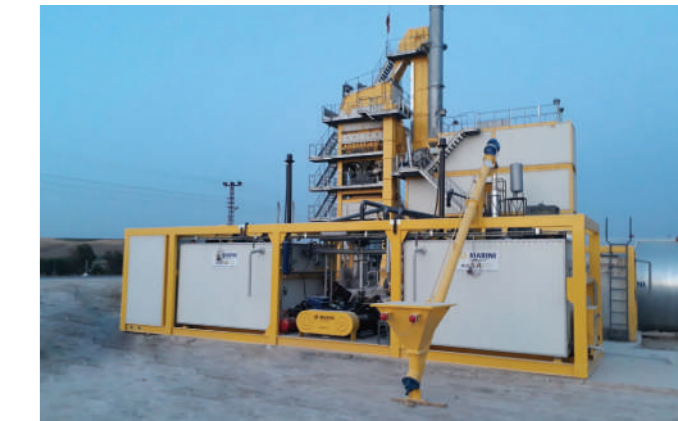
ARGENTINA - modIFALT30 PMB Plant up to 30 t/h
