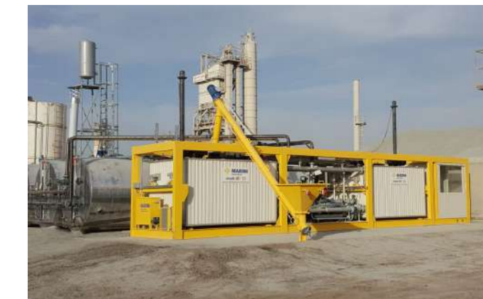
KUWAIT - modIFALT15 PMB plant up to 15 t/h
